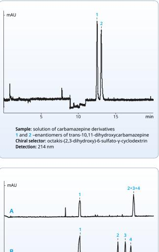
ż ά 5 ģ min Sample: simulated solution 1 - electroosmosis flow of positional isomers of 2 – 4-nitrobenzoic acid nitrobenzoic acid 3 – 4-nitrobenzoic acid A: borate buffer 4 – 2- nitrobenzoic acid B: borate buffer with added Detection: 254 nm **B-cvclodextrin**
